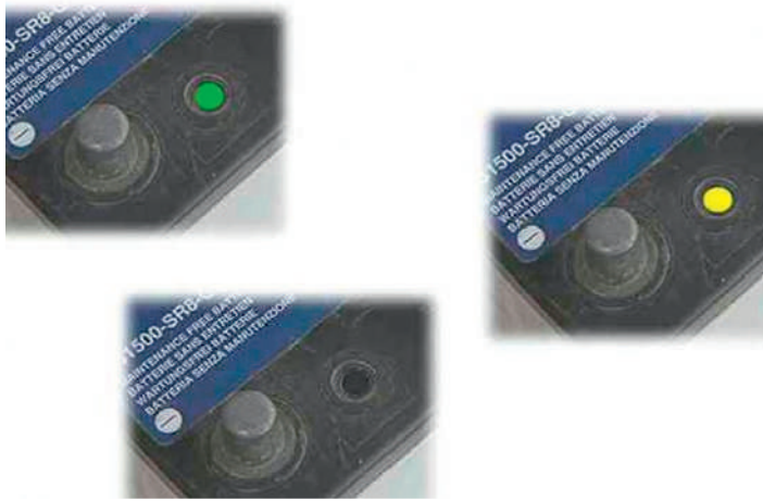
Figure 3.46 Maintenance-free battery hydrometer colours
